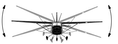
the operation of the ailerons. To roll left, the left aileron is raised and the right aileron lowered. The combined effects of the airflow on the controls lowers the left wing and lifts the right wing. The operation is reversed to roll right.
