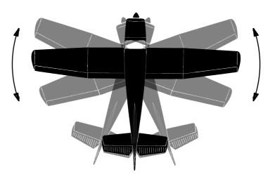
with a sideways motion; it will only turn as a consequence of the secondary effects of controls.
