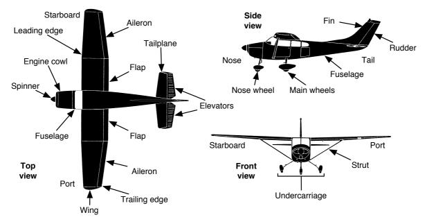
The primary flight controls on any powered aeroplane are: elevator (pitch), aileron (roll), rudder (yaw) & throttle. Gliders have no engine or throttle but their controls are otherwise the same.
